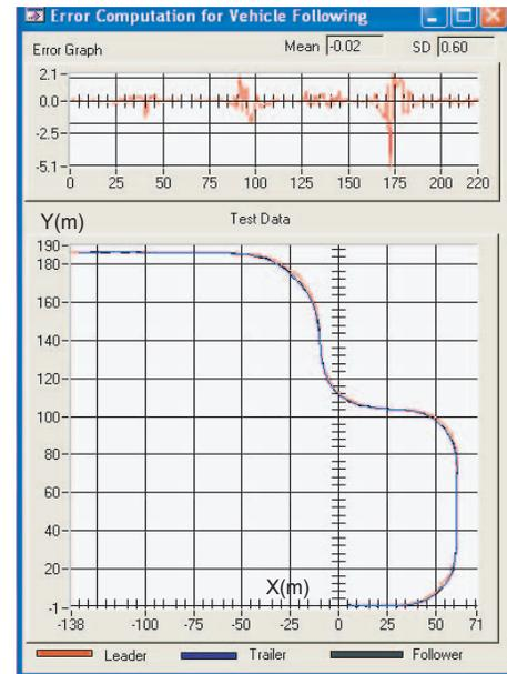
Fig. 9. Test result for vehicle following in urban area. Top graph indicates the tracking error of the follower. Bottom graph shows the trajectories of the leader and follower
