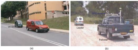
Fig. 8. Experimental setups of vehicle following system in (a) urban and (b) sub-urban environment. Both leader vehicles are travelling at a speed of around 25 km/h (a) along a well paved road and (b) in a jungle. The follower is equipped with on board odometry sensors and a laser scanner.
