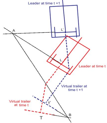
Fig. 5. The leader vehicle moves from  $L$  to  $L'$  (from time step  $t$  to  $t+1$ ), with an instantaneous center of rotation, A. In response, the virtual trailer would have travelled from  $T$  to  $T'$ , with an instantaneous center of rotation B
