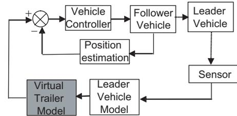
Fig. 3. Control block diagram for the proposed vehicle following system
