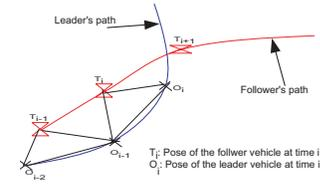
Fig. 7. Computation of tracking errors
