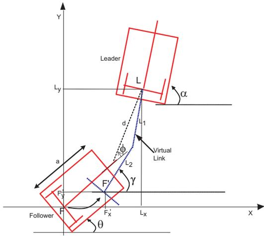
Fig. 4. At any time instance, the follower perceives the pose of the leader with the onboard sensor. The pose,  $F'$ , of the virtual trailer link is then estimated. The follower will be commanded to the new position,  $F'$ . The whole process will be repeated at the next time instance
