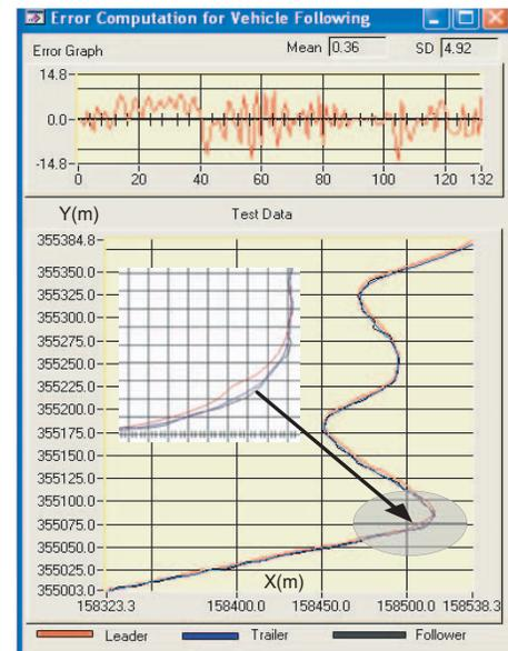
Fig. 10. Experimental result for vehicle following in sub-urban area. The inset image is a zoomed view of the error. Top graph indicates the tracking error of the follower. Bottom graph shows the trajectories of the leader and follower
