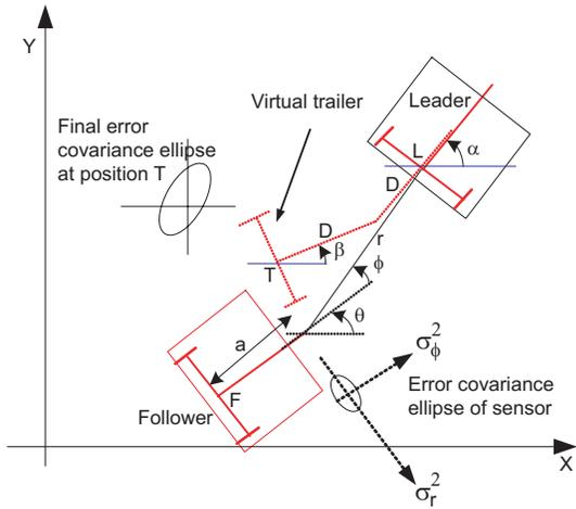
Fig. 6. Demonstration of error propagation. The ellipses indicate the error covariances caused by perception noise. The estimation error of the virtual trailer point is compounded
