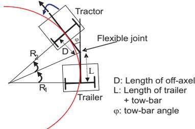
Fig. 2. Off-hooked trailer system under a steady state configuration. Both tractor and trailer are moving on the same circular path if  $D = L$ .
