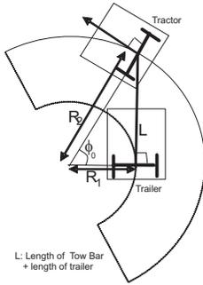
Fig. 1. Direct Hooked Trailer system under a steady state configuration. Both the tractor and trailer are moving on respective circular paths with radii  $R_2$  and  $R_1$  respectively.
